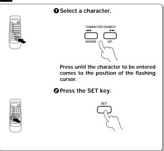
• The characters also can be selected with the **DISC SKIP** knob on the main unit. Turn the knob until the character to be entered comes to the position of the flashing cursor.
